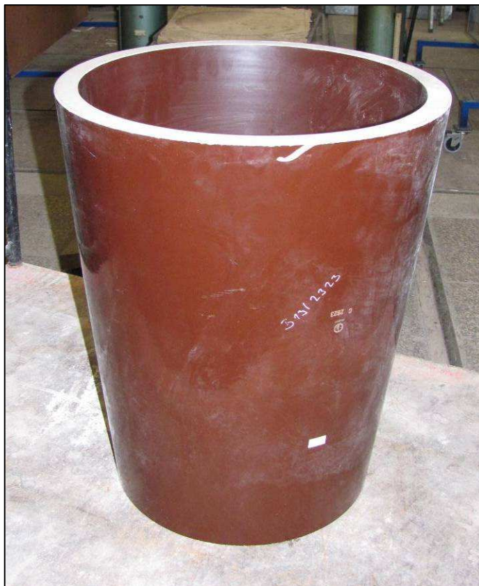
Photo 3: Look at the tested specimen of ceramic electric filter after mechanical compression test – spec. 1/14 (2323)
