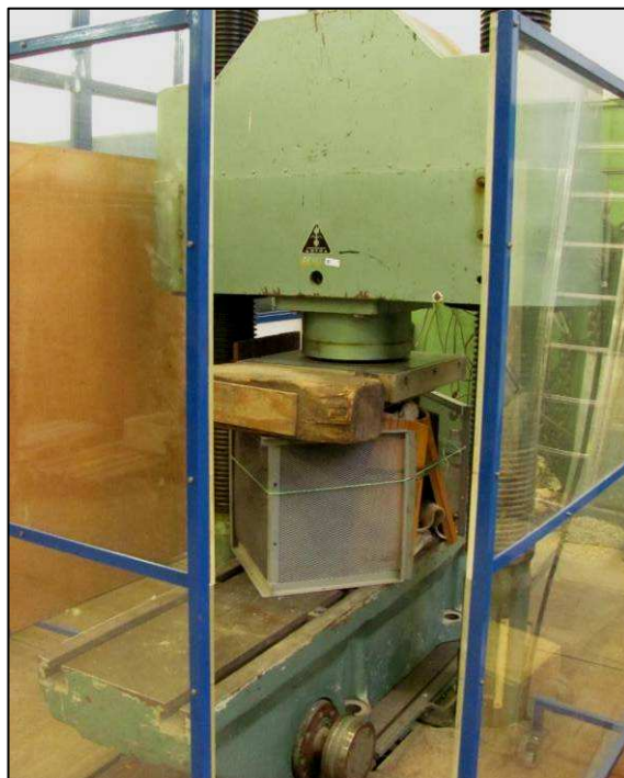
Photo 2: Look at the arrangement of the mechanical test in the compression of the ceramic electric filter
