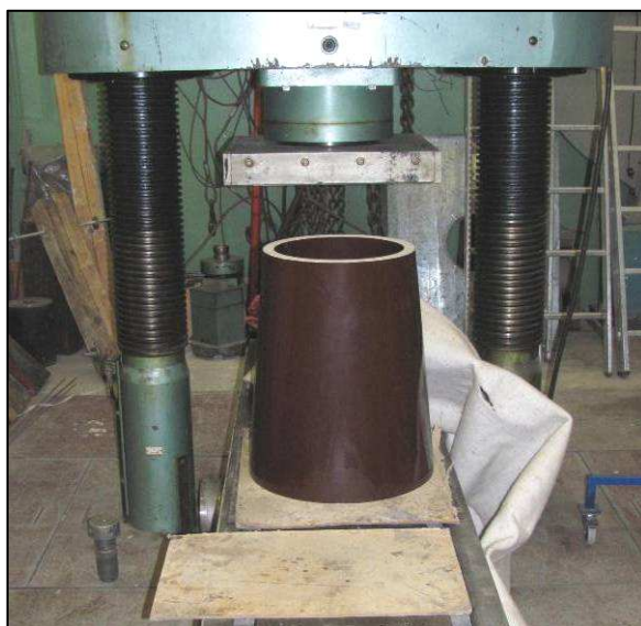
Photo 1: Look at a specimen of ceramic electric filter located in the testing machine
